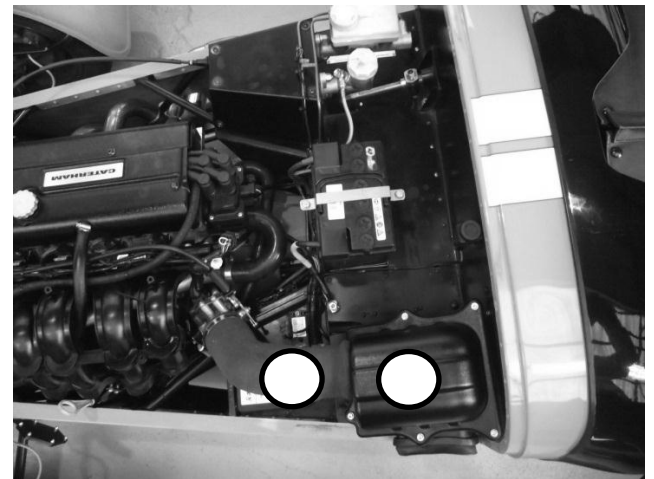
Figure 60: Air intake and trunking
